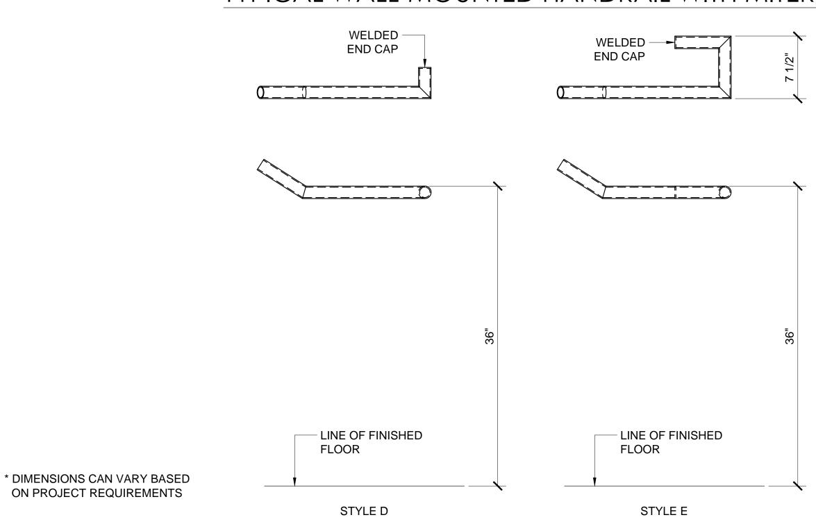
STANDARD WALL RETURN CONFIGURATIONS WITH MITERED CORNERS
