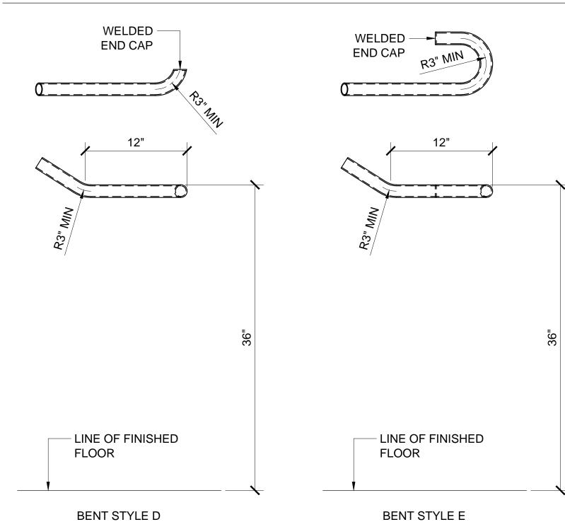
STANDARD WALL RETURN CONFIGURATIONS WITH BENT CORNERS
