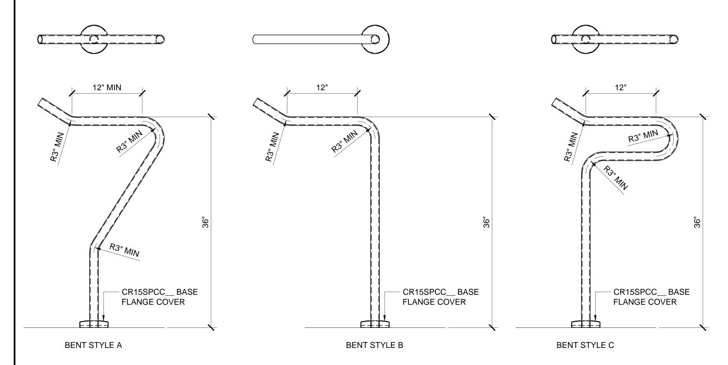
STANDARD FLOOR MOUNT CONFIGURATIONS WITH BENT CORNERS
