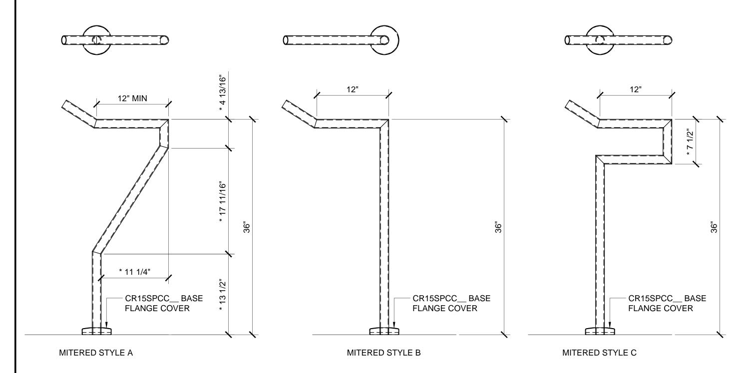
STANDARD FLOOR MOUNT CONFIGURATIONS WITH MITERED CORNERS
